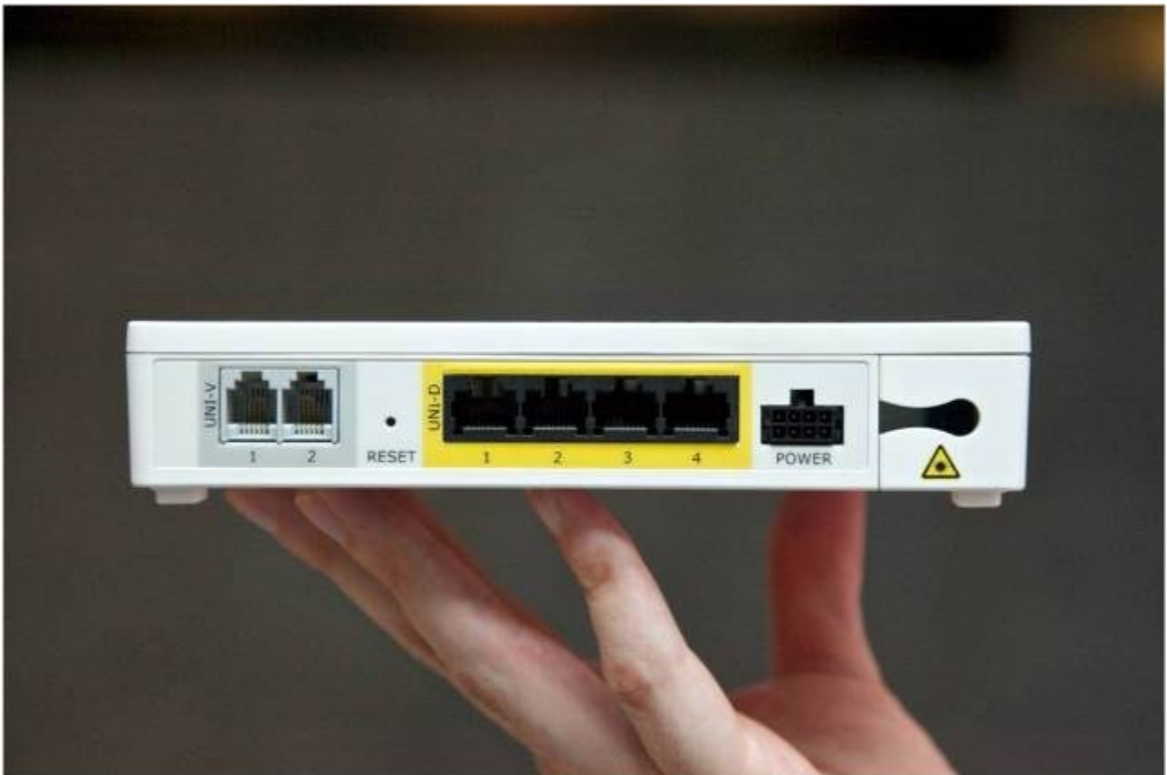
The NBN box has six ports: two phone ports and four data ports. (Courtesy of NBN Co)
