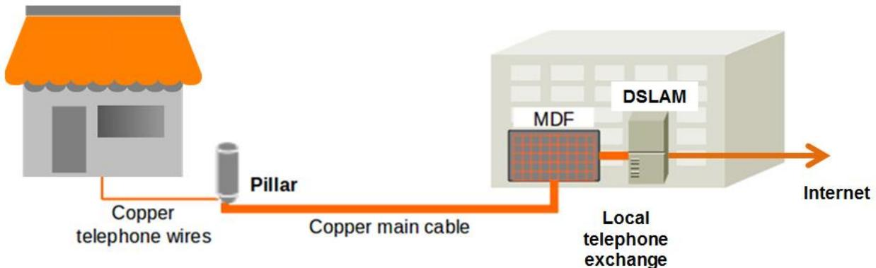
The basic components of a DSL service are a modem on your premises which connects to the main distribution frame (MDF) and then to the service provider's DSL Access Multiplexor (DSLAM).
