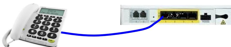
Figure 4 - IP telephone handset connected directly to Ethernet network
